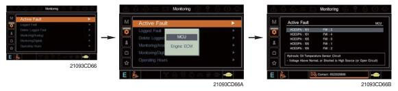
· The active faults of the MCU or engine ECM can be checked by this menu.
